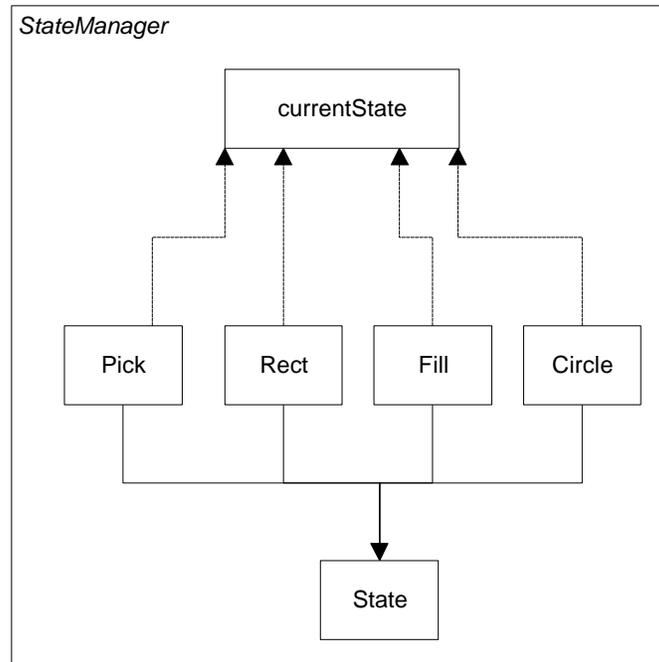
A typical State object simply overrides those event methods that it must handle specially. For example, this is the complete Rectangle state object:
