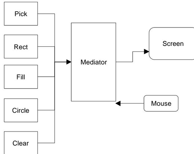
However, this initial design puts the entire burden of maintaining the state of the program on the Mediator, and we know that the main purpose of a Mediator is to coordinate activities between various controls, such as the buttons. Keeping the state of the buttons and the desired mouse activity inside the Mediator can make it unduly complicated as well as leading to a set of *if* or *switch* tests which make the program difficult to read and maintain.
