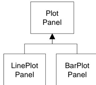
The base PlotPanel class contains the common code for scaling the data to the window.
