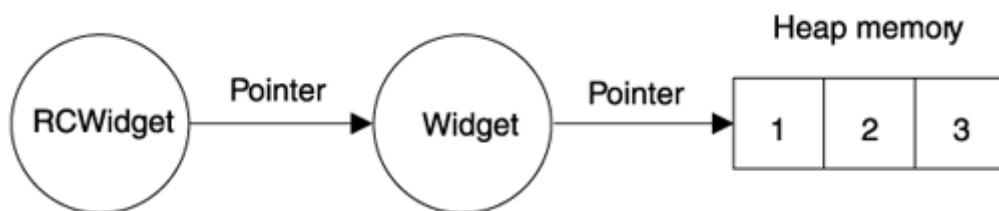
Figure 12.2. A simple design for a reference-counted Widget class.
