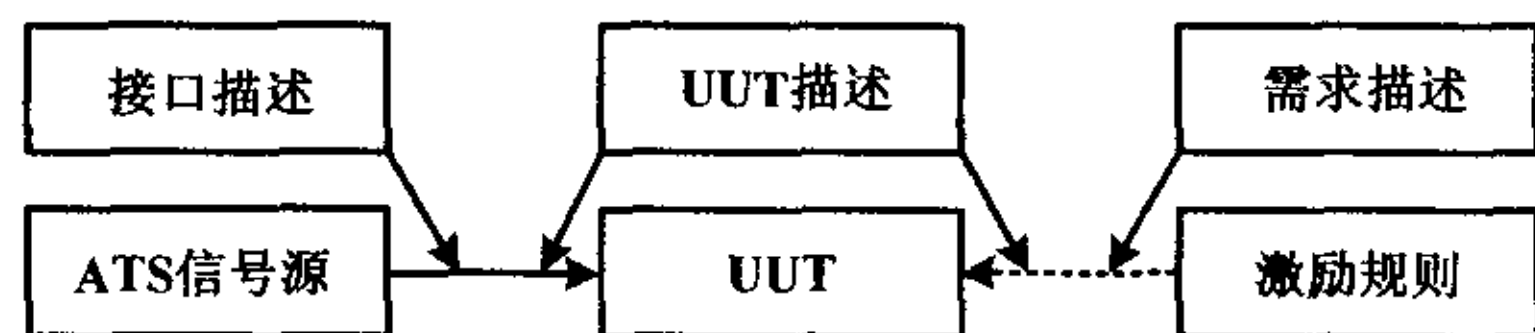
图 4 UUT 信号激励需求问题模式框图及其关注点 Fig. 4 Block diagram of UUT signal energizing demand problem mode and the points to be noted
